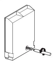
Prise cover loose using screwdriver in position (1) then lever off with screwdriver in position (2) at either side.
